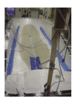
The outer mahogany veneer surface of the hull and deck is created using a unique new production technology exclusively developed by Thore Berntsson. The surface is epoxy coated for maximum strength and durability, before finally being sprayed with two pack polyurethane to give ultimate resistance to ultra violet rays.
